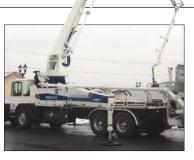
grammable wireless remote control, an LED display delivers feedback through two-way communication. Rexroth Hydraulic pumps and Stiebel PTO create a smooth and quiet pumping operation. Daily maintenance is simplified with the automatic greaser and quick change-out, two-piece-style mud caps. CIFA USA Inc. 877-243-2345. www.cifausa.com.
