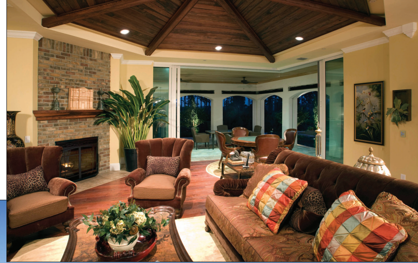
The open floor plan on the first floor combines the main kitchen with an outdoor seating area using telescoping doors. The fireplace features concrete veneer bricks. Photo: Erin O'Boyle Photographics/PCA
